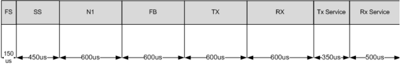
Fig. 3. Frame structure of the implemented MAC.
